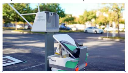
In the coming months, select Wing deliveries will be picked up by a Serve delivery robot from the restaurant's curbside and delivered to a Wing drone AutoLoader a few blocks away, for aerial delivery to customers as much as 6 miles away.
